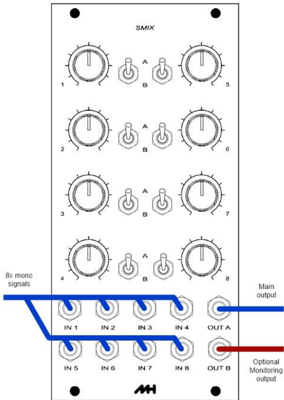
Here we are mixing up to 8 mono channels. All the selector switches are set to 'A' so the full mix is available at OUT A. If any channel is switched to 'B' that channel will appear at OUT B, so this can be used as a 'preview' facility. Typically, OUT B might feed a headphone amplifier so that sounds can be checked / adjusted before being added back to the mix by switching the relevant channel to 'A'.
