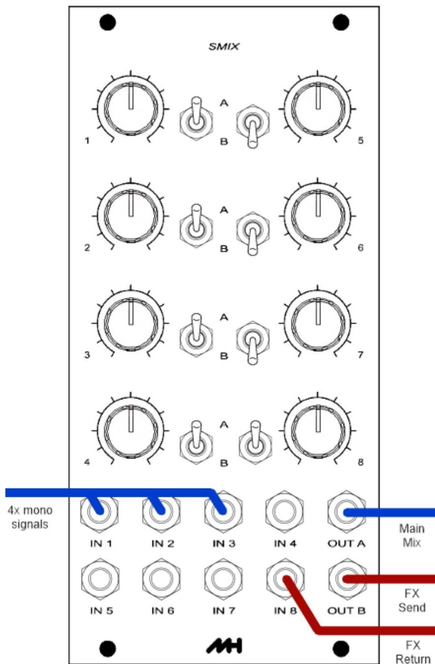
This is a variation of the previous example which brings back the FX return into channel 8. The channel 8 switch is now set to 'A' and the level control for this channel is now the FX return level. Channel 4 no longer has an associated FX send but can still be used as either a 100% dry input (switch to 'A') or 100% wet input (switched to 'B').
