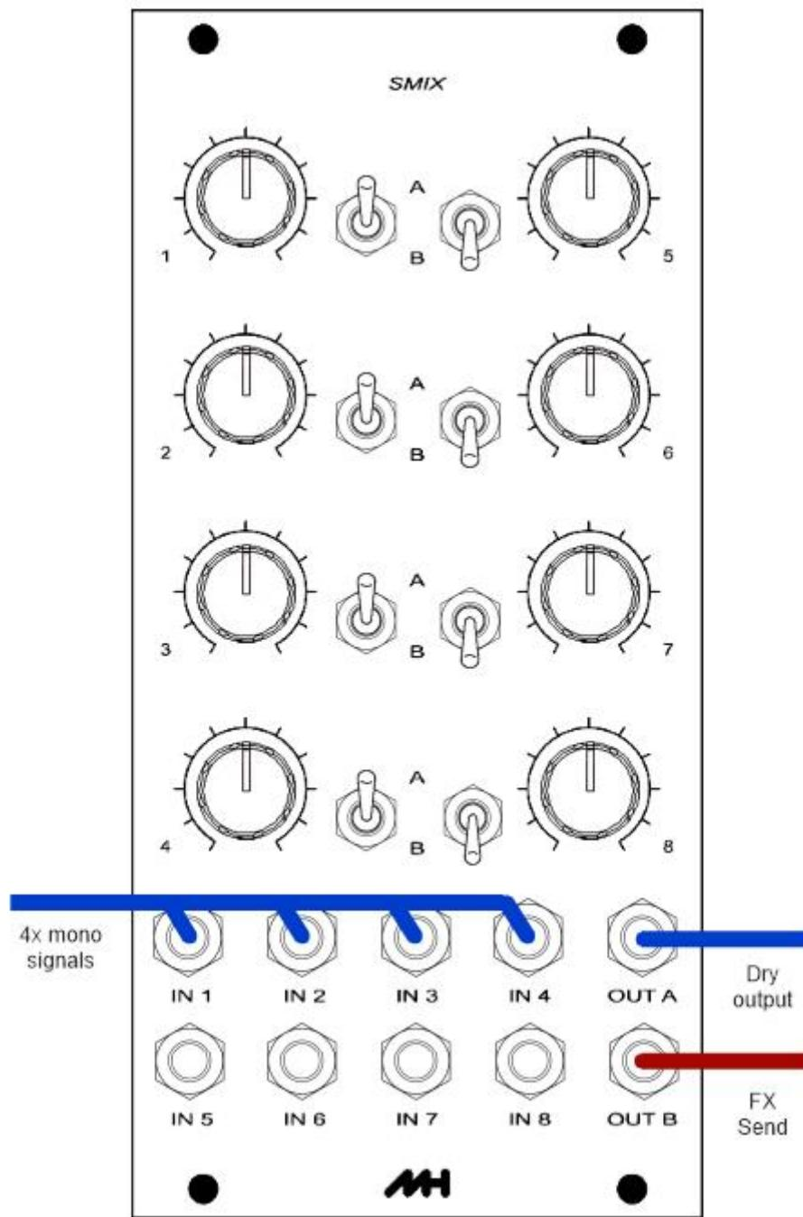
Here we utilise the channel normalisation to copy the signals plugged into channels 1 to 4 over to channels 5 to 8. Channels 1 to 4 are switch to 'A' and the dry mix is available at OUT A. Channels 5 to 8 are switch to 'B' feeding the FX send mix at OUT B.
