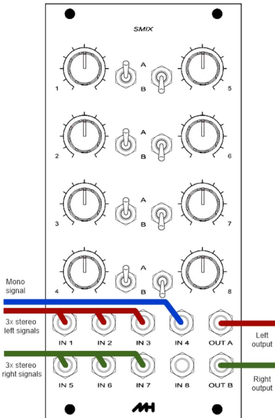
For stereo mixing select 'A' on channels 1 to 4 and 'B' on channels 5 to 8. Left or mono signals can be routed to channels 1 to 4, with right signals going to on channels 5 to 8. With the SMIX input normalisation, mono channels will appear on both left and right outputs.
