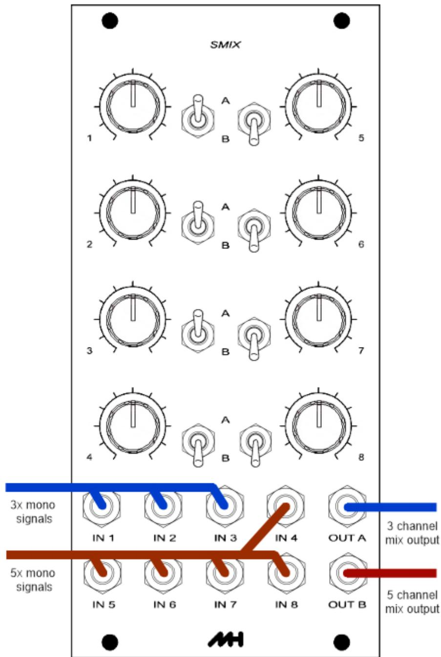
SMIX can be configured as two separate mono mixers. The above diagram shows a 5-3 channel split, but 6-2 and 4-4 splits are also possible. For this example, channels 1 to 3 are switch to 'A' with their mix available at OUT A. Channels 4-8 are switch to 'B' with their mix available at OUT B.
