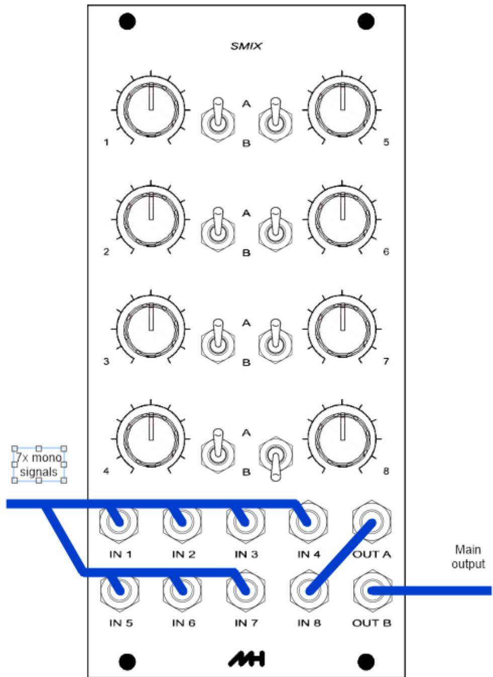
With one less channel we can have a master level control. All the selector switches are set to 'A' with the exception of channel 8 which is set to 'B'. OUT A is patched to IN 8 and the mix is available and OUT B with the level control for channel 8 acting as a master level control for the entire mix.
