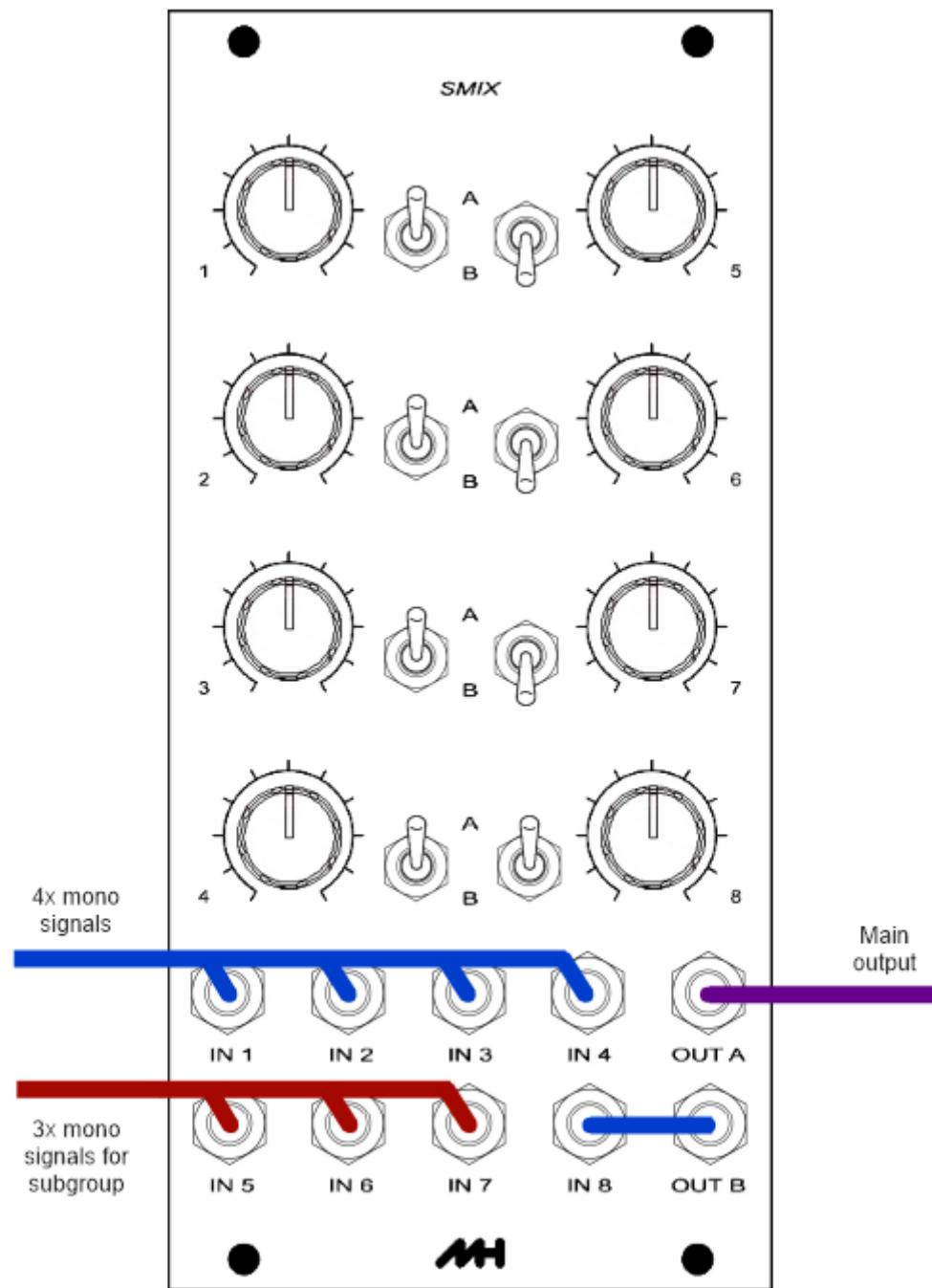
Sometimes it's useful to control the level of a number of channels simultaneously. For example: the level of all the drums/percussion in a mix. In this example we have the inputs 5 to 7 grouped together. They are all switched to 'B' and OUT B is patched to IN 8 which allows the level of all 3 channels in the sub group to be altered by the channel 8 level control.
