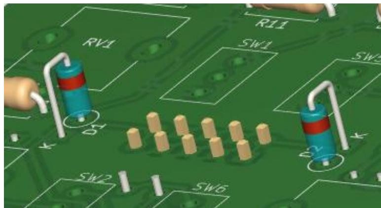
Turning to the other side of the board (the side with the MH logo), place and solder resistors R5 to R10 and R13 to R26. Note these are different values – Check BOM
